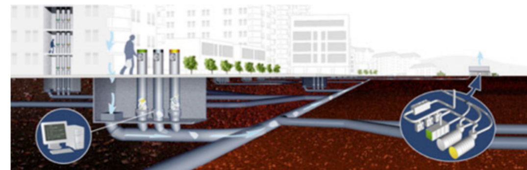
Model of the waste disposal system.
