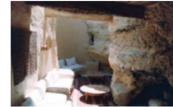
Fig (8.4): The buildings carved into stones with thick walls creates cool areas
